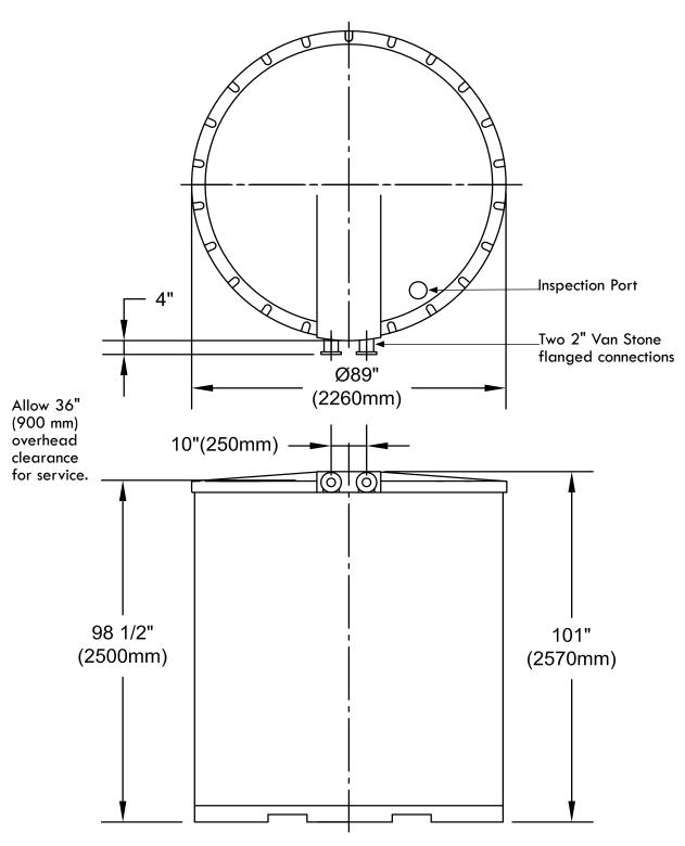
**NOTE:** Tolerance for all dimensions is  $\pm$  1/2" (12.5 mm)
